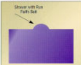
FIGURE 6: With slow oscillation, the cut made on the return stroke will remain in the cut made on the forward stroke for an extended period of time.
