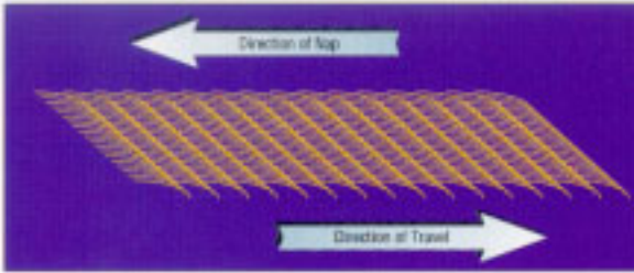
FIGURE 4: A jet directed into the run will tend to densify and part the nap.
